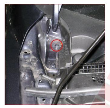
Position the mirror above the rear mounting bolt of the bonnet stay with the mirror facing upwards.
